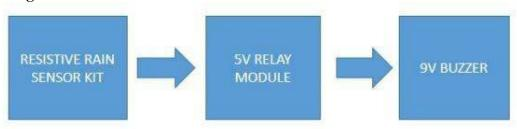
Block Diagram Explains the working of Rain detector alarm
