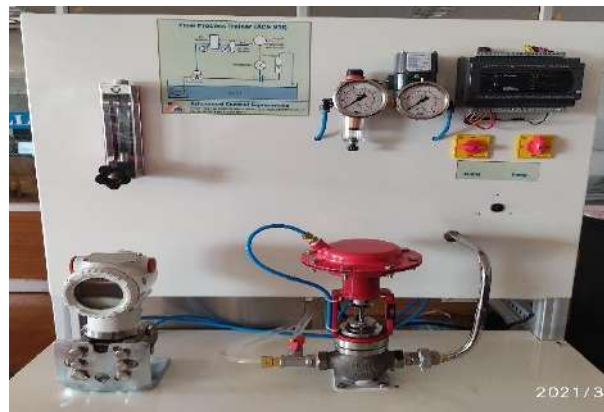
Fig 1: Experimental setup for flow monitoring and control system
