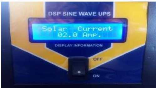
Fig.14 Solar current obtained in solar priority
