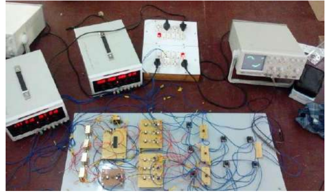
Fig.10. Hardware implementation of single H Bridge MLI
