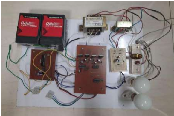
Fig:12 Prototype model of single phase inverter with arduino-ATMEGA 328 based PR controller
