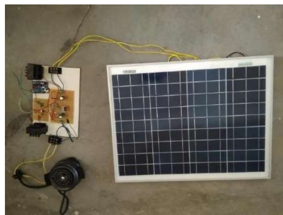
Fig 10: Hardware design of solar powered DC electric heating stove
