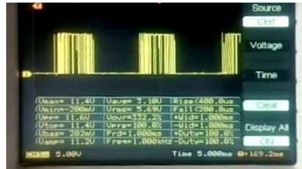
Fig. 9 Positive half cycle on High-side MOSFETs
