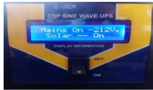
Fig.15 Grid voltage obtained in grid priority
