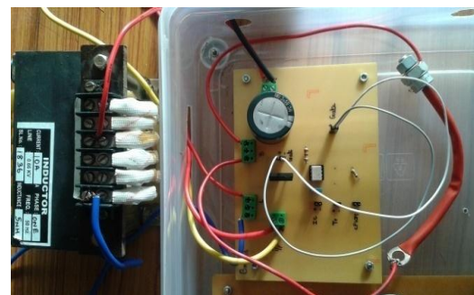
Fig. 2b. Experimental setup of Boost Converter
