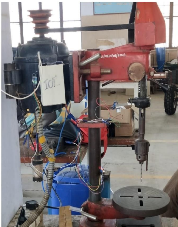
FIGURE 1: Global Monitoring of Bench Drilling Machine using IOT
