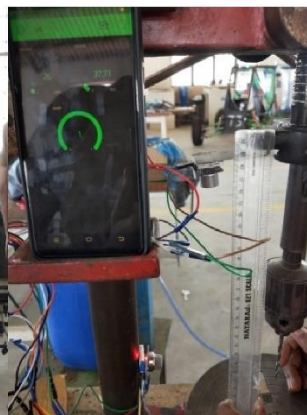
FIGURE 2: Monitoring of Bench Drilling Machine via Android Platform
