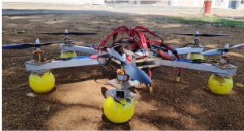
Prototype model of the Air pollution Monitoring- Drone
